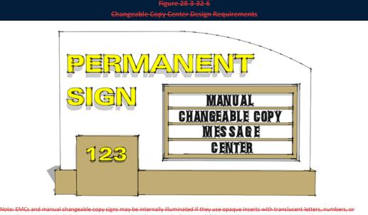
lote: EMCs and manual changeable copy signs may be internally illuminated if they use opaque inserts with translucent letters, numbers, o ymbols, as displayed by "A" above. These signs shall not be internally illuminated if they use clear or translucent inserts with opaque or ranslucent letters, numbers, or symbols, as displayed by "B" above.
