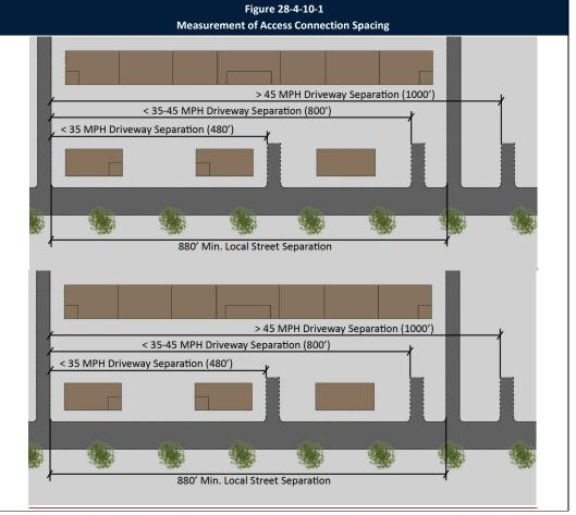
A-I. Access Spacing, Opposite Sides of Street. In order to prevent conflicting left-turn movements, connections on opposite sides of <a href="mailto:the-streetcollector">the-streetcollector and arterial streets</a> shall be directly opposite each other or offset by a distance of at least 75 feet, unless a median prevents the potential conflicts.
